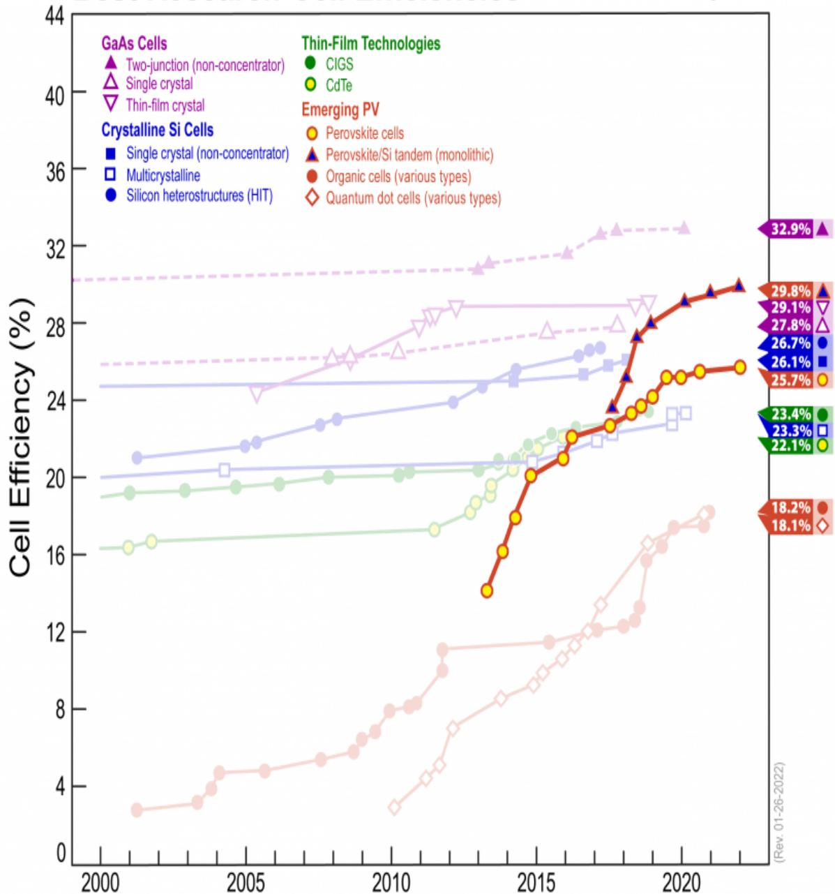
Efficiency records for perovskite PV cells compared to other PV technologies, with current records of 25.7% for single junction perovskite devices and 29.8% for tandem perovskite-silicon devices (as of January 26, 2022).
